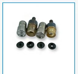
In order to complete the products you have designed as you imagine, you can easily use the 10,5 mm plastic snap fateners fastening mold (assembly mold) in mass production, small-scale works or for hobby purposes, and you can assemble it as you wish. When
